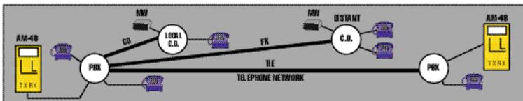
Use the AM-48<sup>XT</sup> built-in dial capability on dial-up networks to access a second AM-48<sup>XT</sup> for centralized 2-wire testing.
