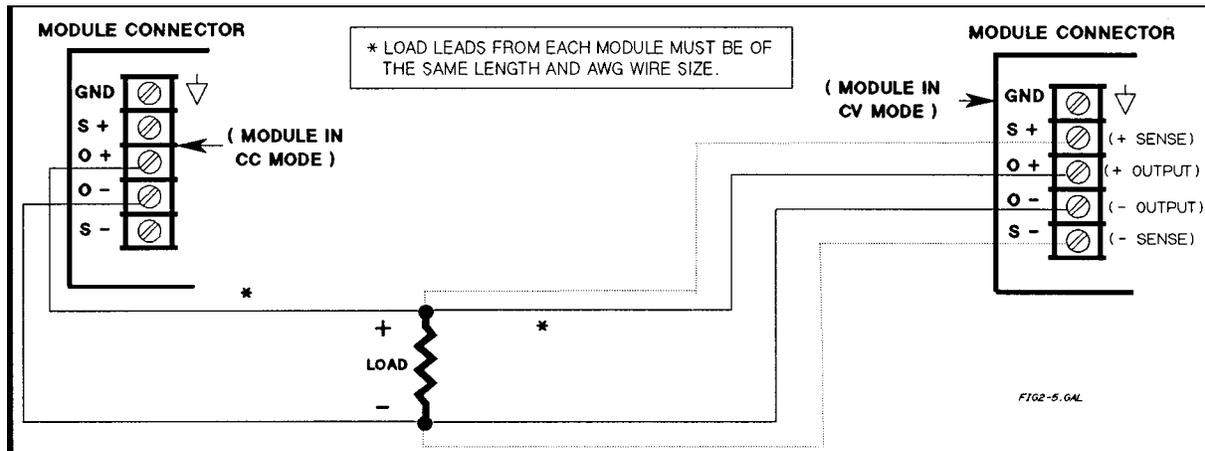
Figure 2-5. Connecting Power Modules in Parallel
