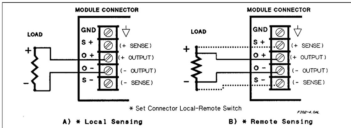
Figure 2-4. Load Connection
