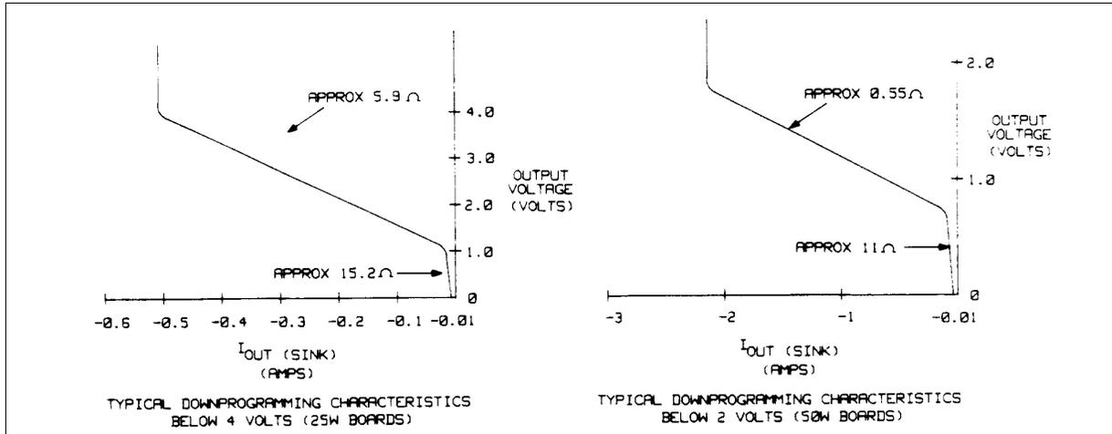
**Figure 4-3. Typical Downprogramming Characteristic Below 2.0 V**
