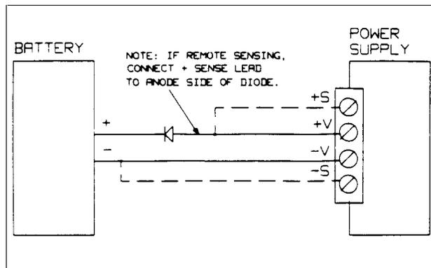
Figure 4-10. Recommended Protection Circuit for Battery Charging
