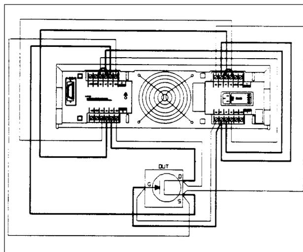
**Figure 4-15. Bipolar Operation**
