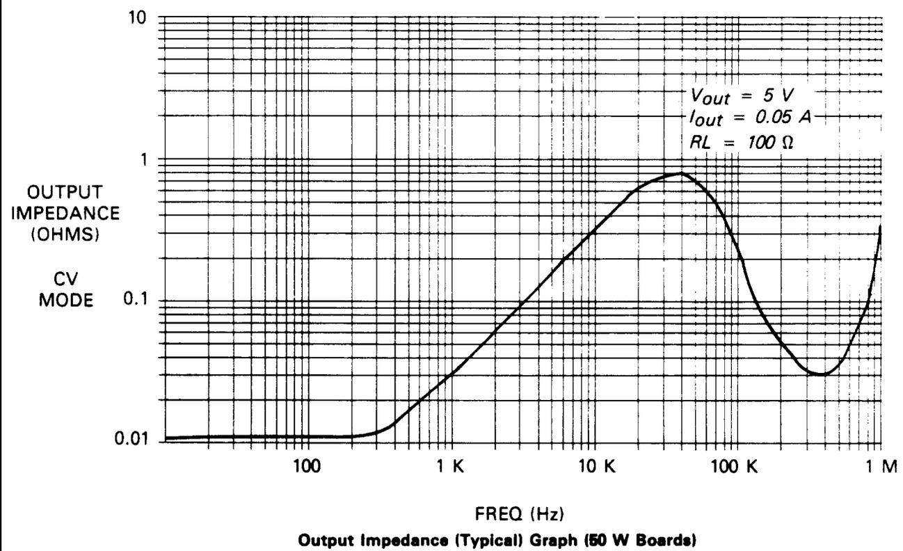
Figure 1-7. Output Impedance (Typical) Graph (See Supplemental Characteristics)
