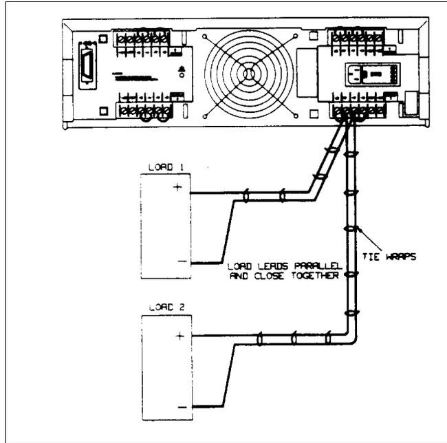
**Figure 4-4. Optimum Hookup for Multiple Loads, Local Sensing**
