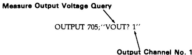
When you send a query from remote, the supply does not display the response as it did when you executed the command from the front panel. Instead, it holds the response in an output buffer. The output buffer is a register that holds information until it is read by the computer or is replaced with new information.
