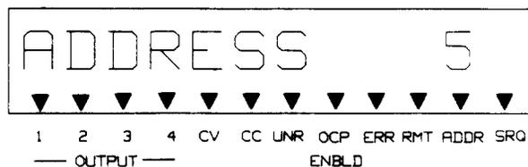
**Figure 3-3. Typical Address Display During Power-On Self Test**
