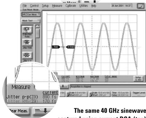
The same 40 GHz sine wave captured using current DCA (top) and now with 86107A precision timebase module (bottom).
