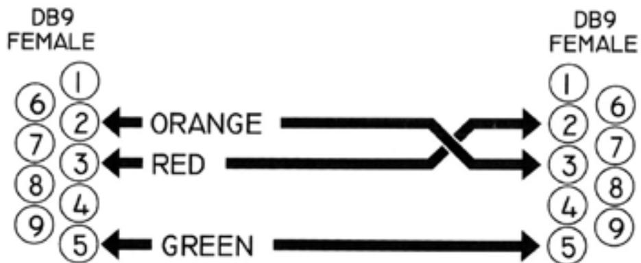
When connecting the TravelPilot to your computer, if a gender changer is needed, it cannot be pin-for-pin. The Rx and Tx lines need to be crossed (as shown in the diagram). Some manufacturers of gender changers will connect pins 1-9 to pins 1-9 directly. The lines need to be connected as in the diagram. Otherwise, you will not be able to communicate to the TravelPilot.
