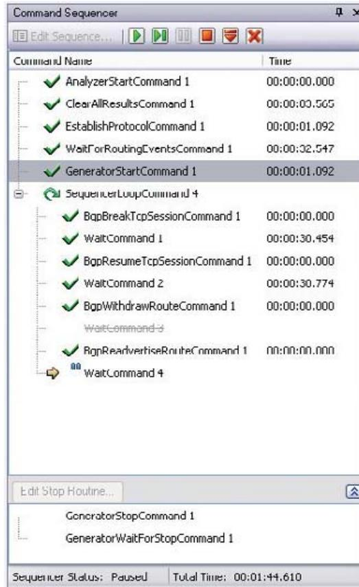
Users can create detailed and automated control over test events using the command sequencer.
