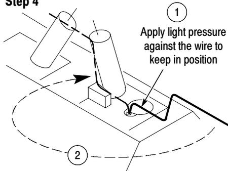
Pivot wire to position it on top of the support block. Then use flat blade end of adjustment tool to push wire down between block and probe tip.
