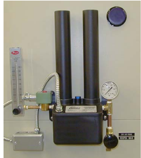
Heatless Desiccant Dryer
